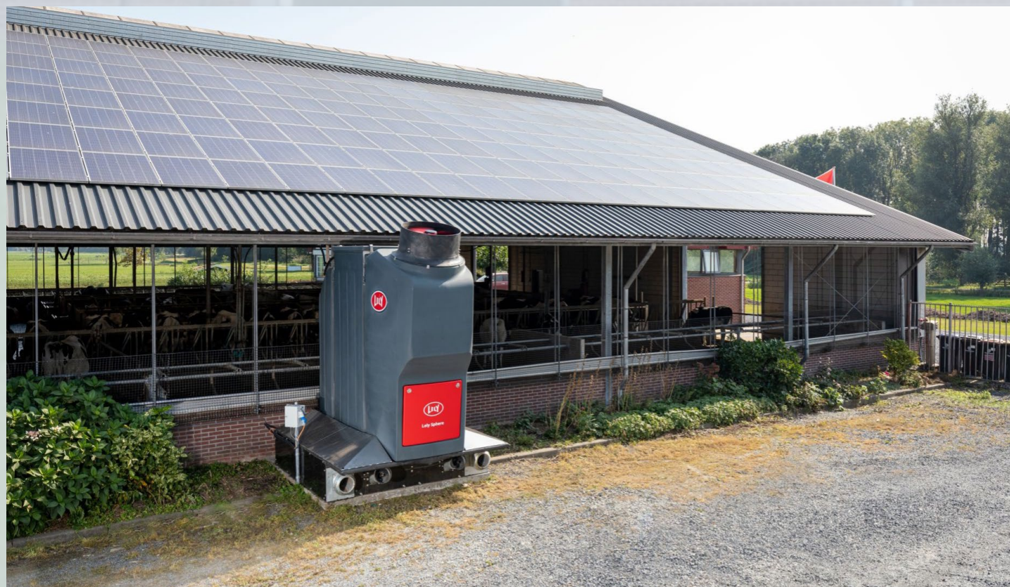
Figure 2: The Lely Sphere N-Capture extracts the manure gases in the cellars and just above the barn floor. The filter package in the N-Capture captures the ammonia and converts it, using water and acid, into circular fertiliser.
