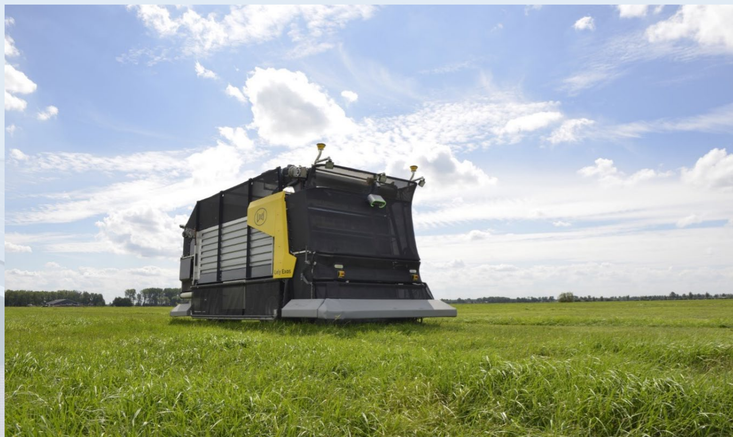
Figure 5: The Lely Exos concept is the first system in development for autonomous harvesting and feeding of fresh grass.
