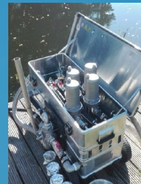
Figure 2: Microplastic sampling system; the 'Rocket' (Foto: Robin Lenz).
