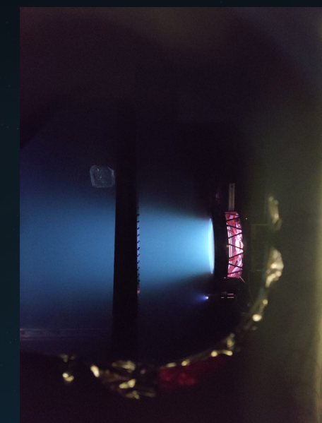
Figure 4: RIT-2X thruster under operation within coupling test.
