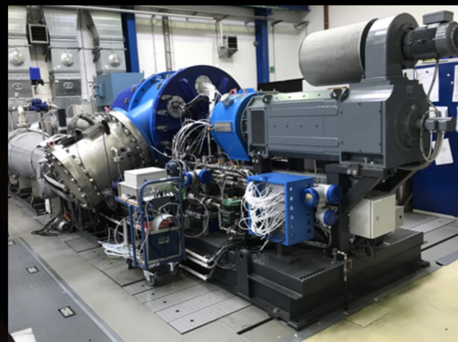
Figure 9: Centrifugal compressor stage test rig at IKDG of RWTH Aachen University.
