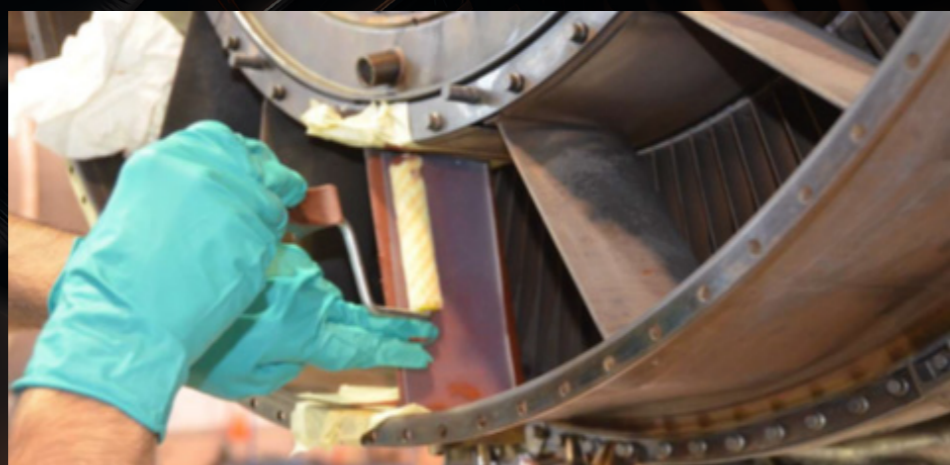
Figure 6: Riblet application with silicone mould
