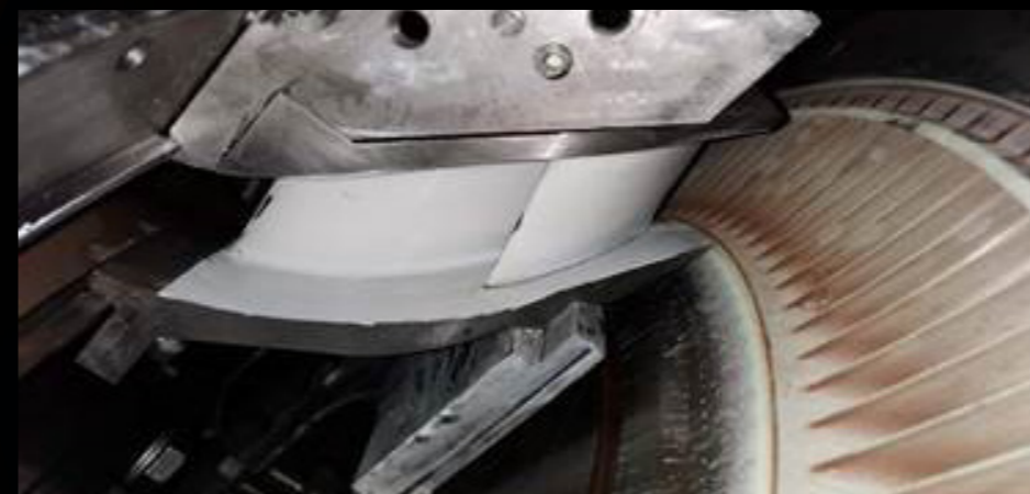
Figure 7: Riblets applied on the airfoils of Pilot 1 at Graz University of Technology.
