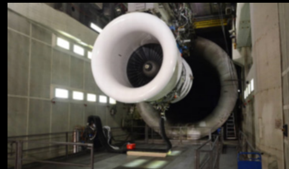
Figure 3: Test engine installed in an engine test cell.
