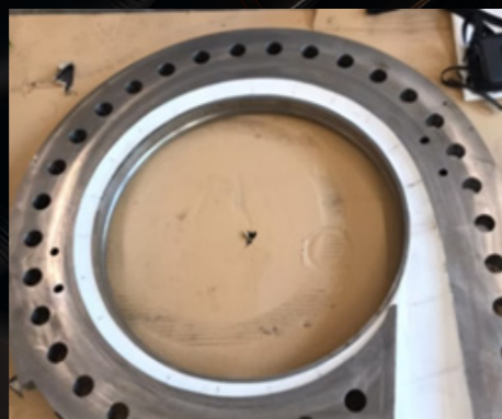
Figure 10: Riblet application on the volute of the centrifugal compressor, Demonstrator 2.
