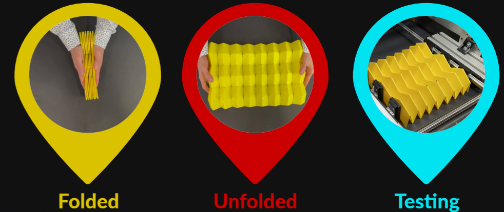
Figure 2: The S-FOAM project develops self-foldable materials using origami and kirigami principles, enabling adaptive folding in response to stimuli, without predetermined lines or advanced electronics.
