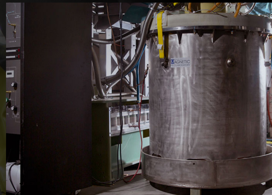
Figure 3: 75 T pulsed duplex magnet made of two nested coils, each independently powered by its own capacitor bank. Developed at the MagLab's Pulsed Field Facility. Credits: MagLab LANL.
