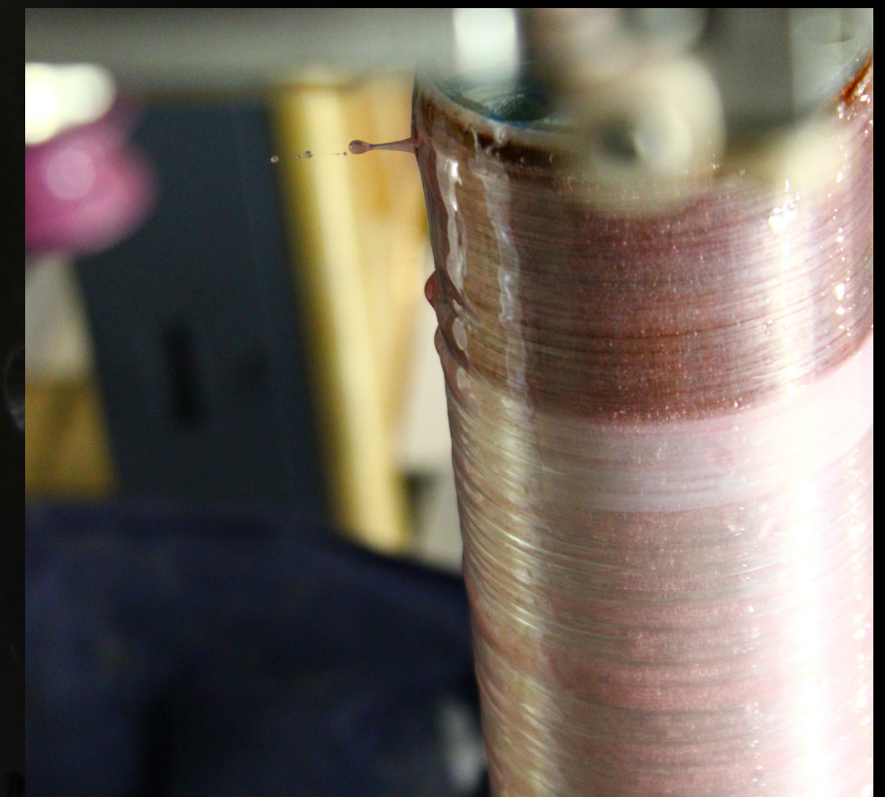
Figure 1: Carefully wound coil wires form the core of a pulsed high-field magnet, essential for producing stable and powerful magnetic fields in experiments. Credits: Kim Schneider and MagLab LANL.
