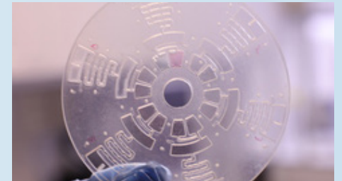
Figure 1: One of the microfluidic devices developed by the team, based on a non-traditional microfluidic design.
