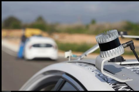
Image: SELFY vehicle demonstrator with LIDAR during real-world demonstrations
