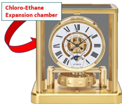
Figure 3 ATMOS clock – chloroethane is used due to its X10 larger vapour pressure sensitivity to temperature variation.
