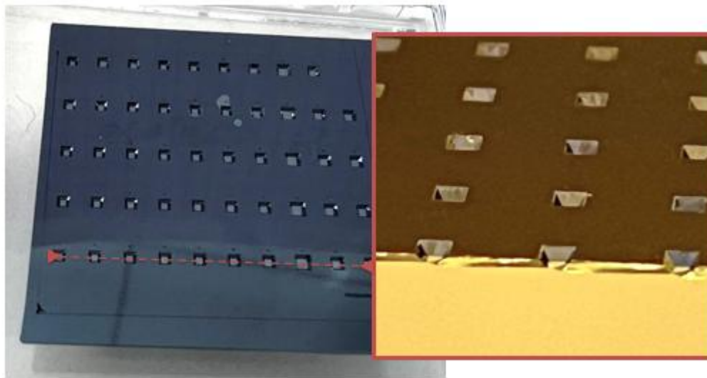
Figure 5. Fabricated chambers with released membranes.
