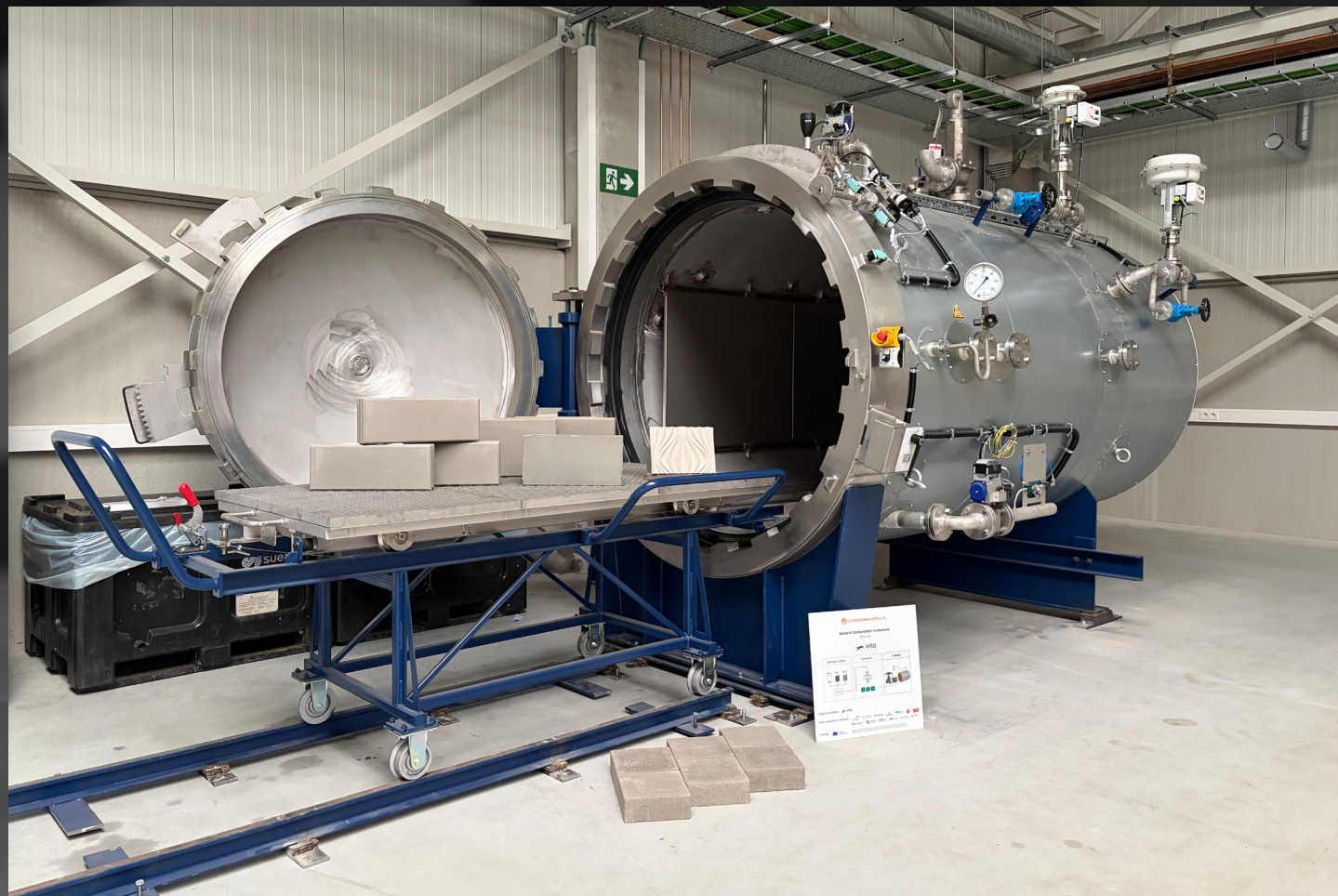
Mineral Carbonation Autoclave Pilot 4b in VITO.
