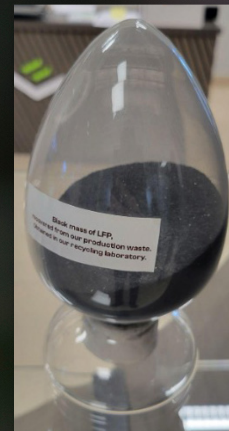
Figure 1: Lithium iron phosphate (LFP) black mass recovered from ElevenEs production waste, obtained in ElevenEs recycling laboratory.
