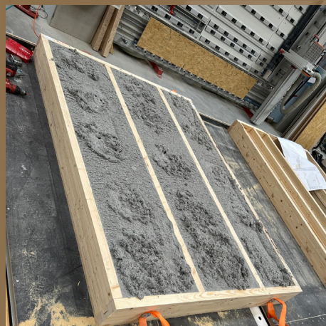
EcoTechWall – North European type with recycled wood and cellulose insulation.
