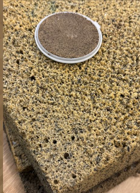
KARZ – insulation material made primarily from coffee grounds.
